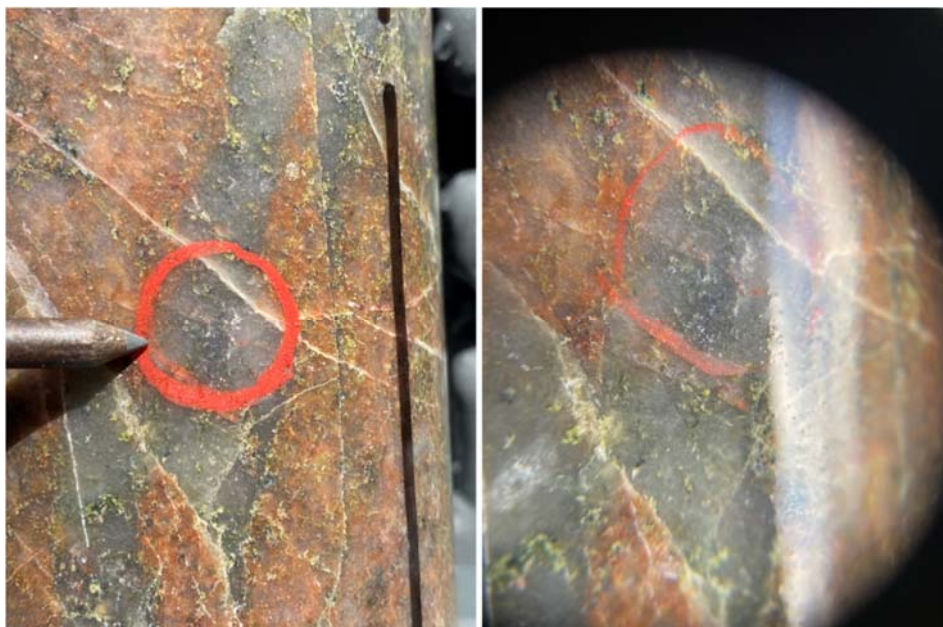
Figure 8: Quartz + pyrite + molybdenite bearing vein.
