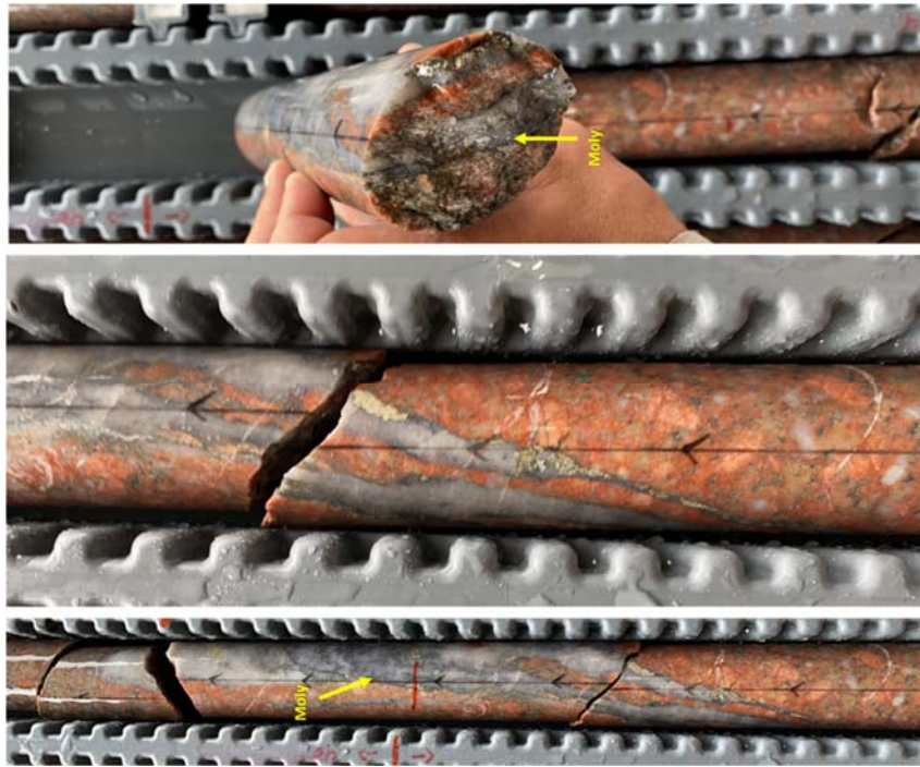
Figure 7: Quartz + pyrite + molybdenite bearing vein.
