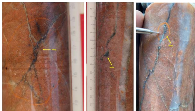
Figure 6: Molybdenite filling fractures.
