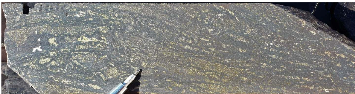
Plate 1c: VUD0019 - 1416.1m. Layered chalcopyrite and lesser pyrite mineralisation in hematite breccia. NQ2 ½ core.
