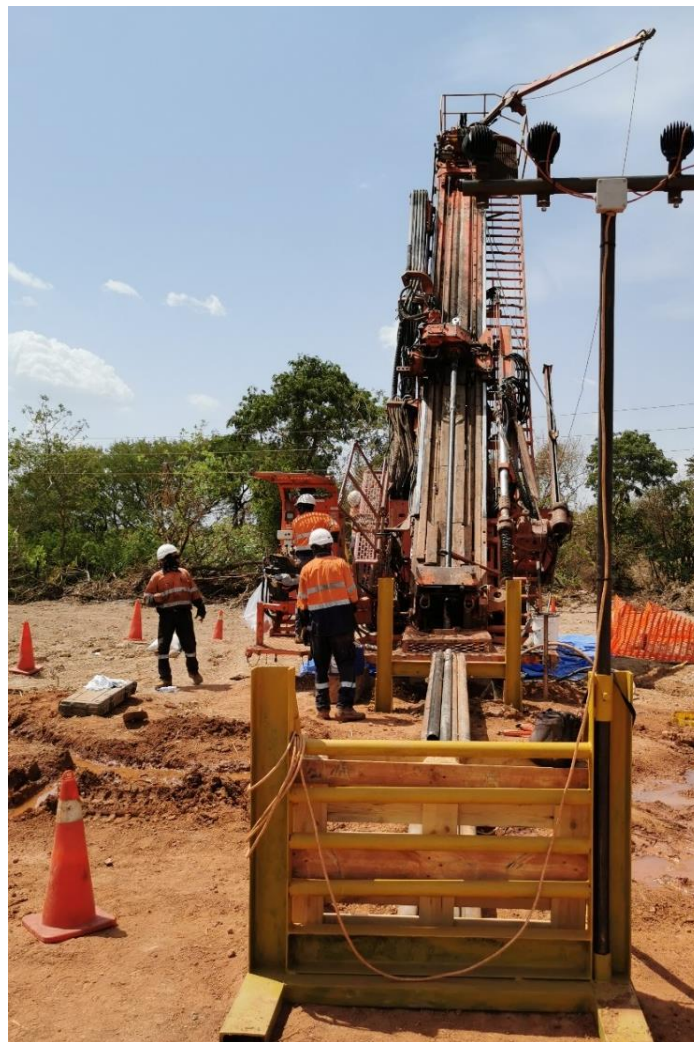
Figure 4. Diamond core drilling at Morila.
