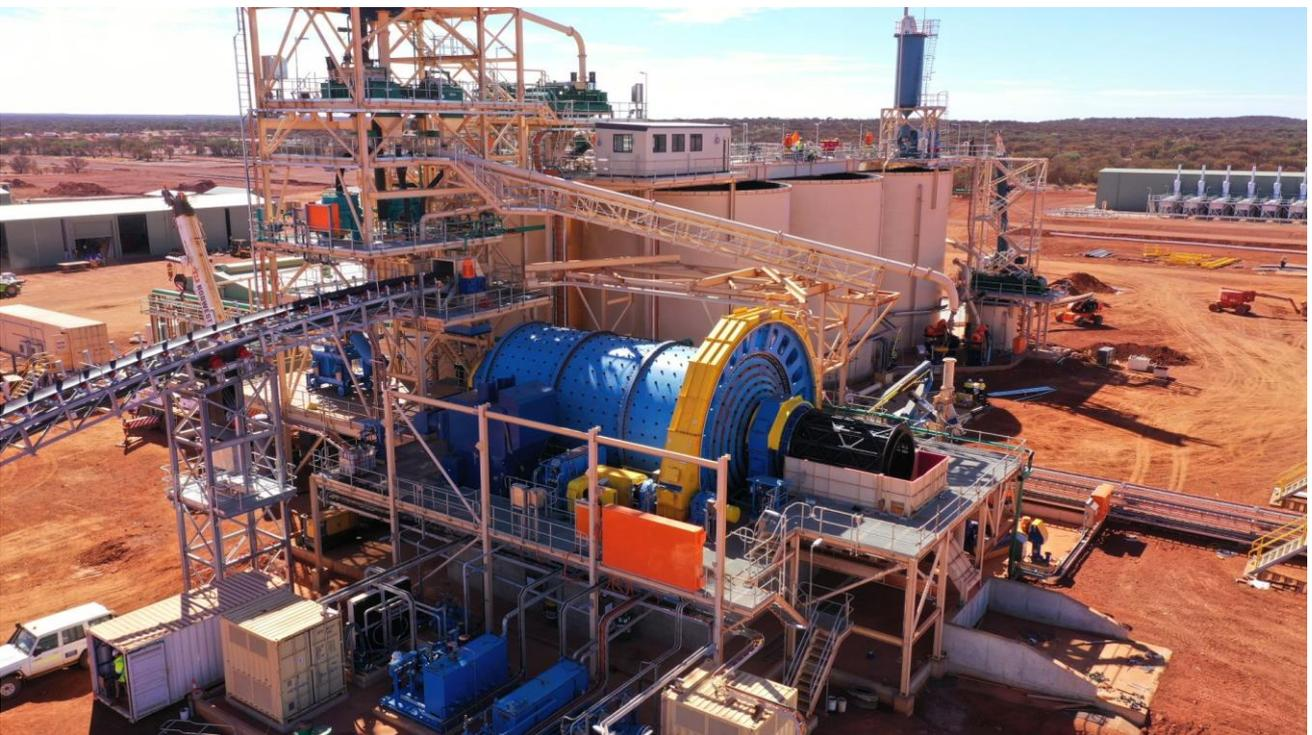
7.5MW ball mill installed aligned and fully rubber lined. VSD motor commissioning underway.
