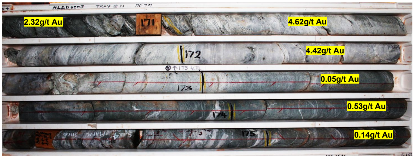
Figure 2 – Assays shown over part of the main mineralised zone at Lily Albany, with assay results quoted on a metre by metre basis (e.g. 171-172m recorded 4.62g/t Au). showing strong alteration and shearing of the host Layered Mafic Complex dolerite, with intense quartz-sericite-pyrite-chalcopyrite alteration evident (ALAD0002, tray #31, 170.7 – 175.35m).
