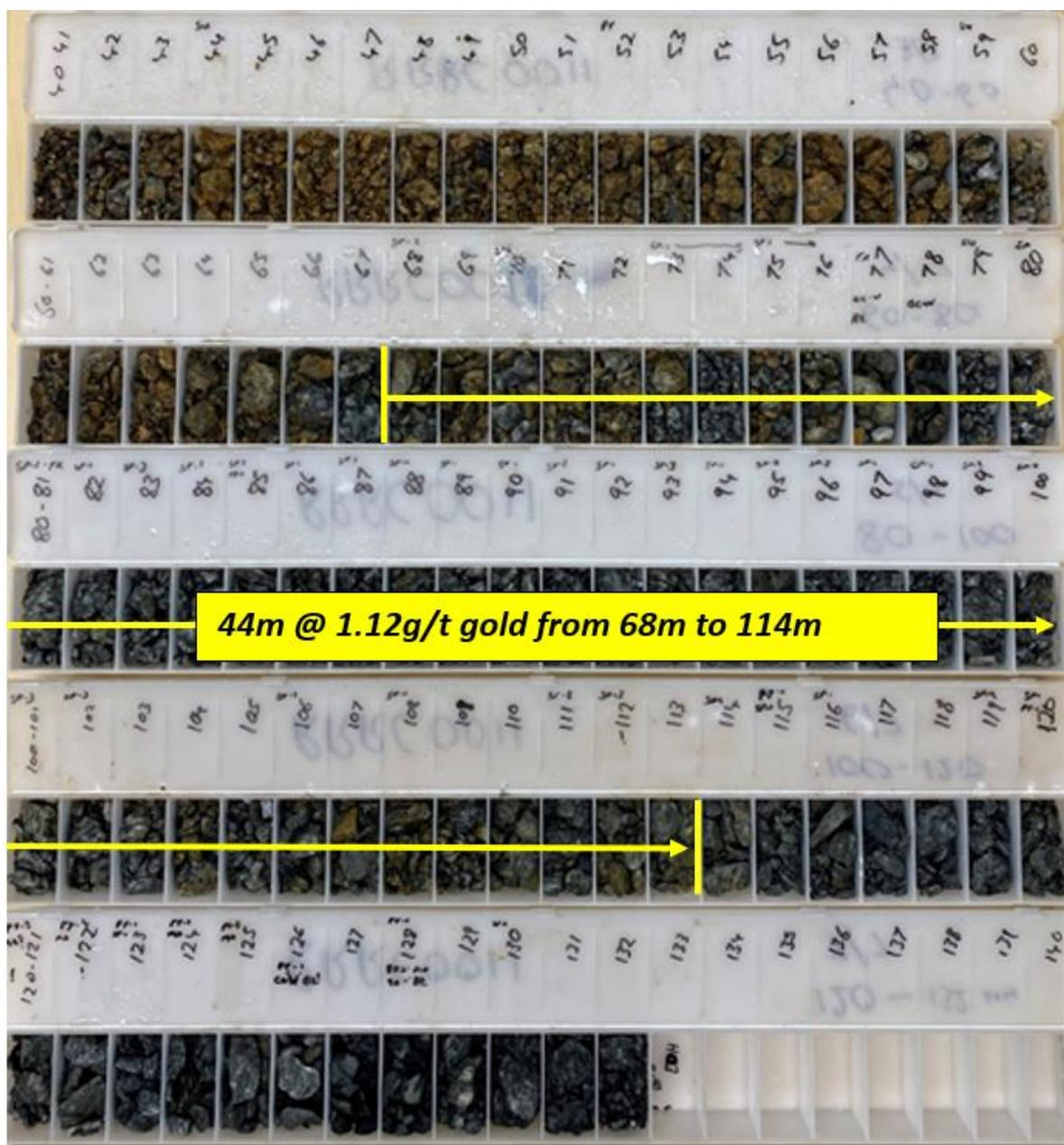
Figure 3; RC chips from RRRC0011
