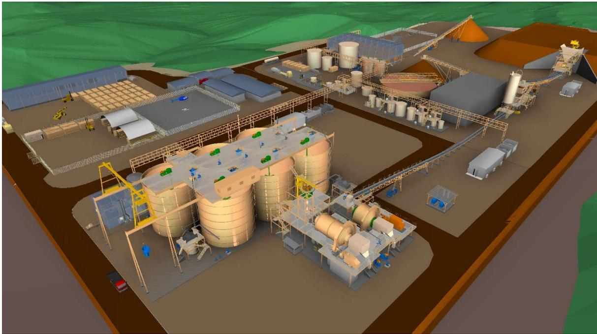
**Figure 1. Redesigned Stage 1 circuit incorporating provision for possible future expansion.**
