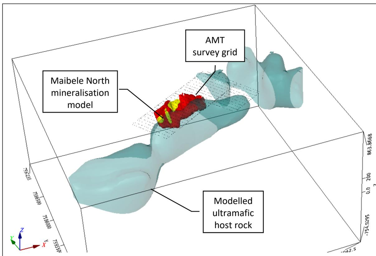
Figure 2. 3D, oblique view of the interpreted Maibele North ultramafic body with ore zones and survey design
