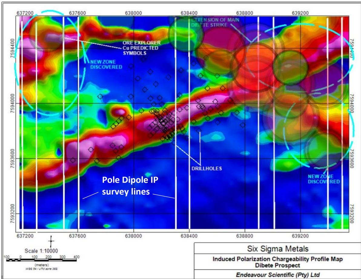
*Figure 4. Dibete - proposed pole-dipole survey lines (white) over gradient array IP chargeability anomaly map with AI-generated target zones (circles)*
