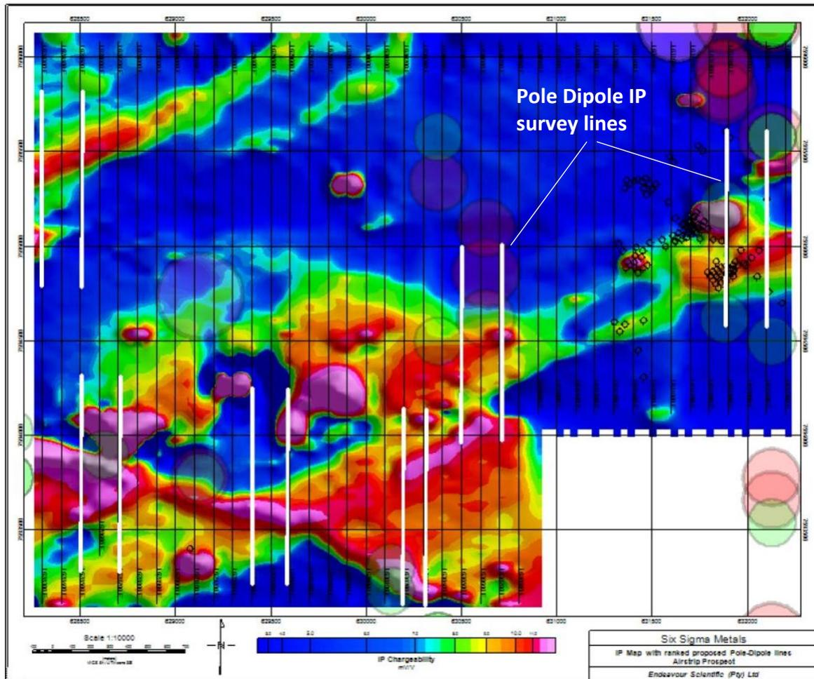
Figure 3. Airstrip - proposed pole-dipole survey lines (white) over gradient array IP chargeability anomaly map with AI-generated target zones (circles)
