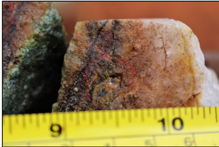
Photo 2: Claypan: Visible gold in BBDD0105 at 78.9m (within 1.54m @ 3.56g/t Au from 78.46m)
