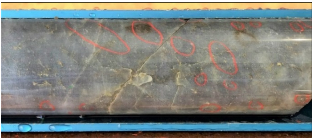
Photo 1: Bombora: Typical silica-albite-sulphide Tura Lode mineralisation in BBRD1135 at 246.70m (assaying 184.64g/t Au); Multiple clusters of fine visible gold are circled in red; Core diameter is 47.60mm
