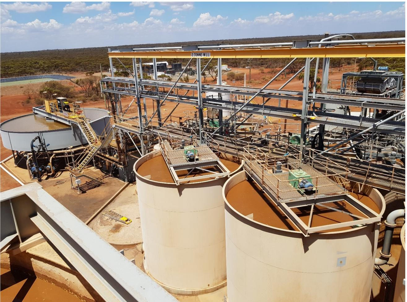
*First commissioning feed through adsorption tanks with tails to thickener*
