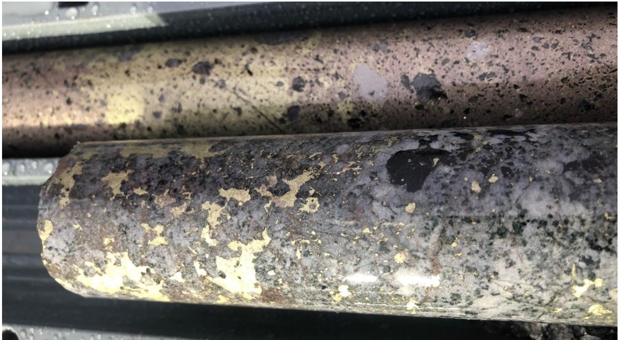
Figure 9: 21PHDD002 Coarse-grained disseminated chalcopyrite and pyrrhotite in foreground and massive chalcopyrite and pyrrhotite with lesser arsenopyrite in the background.
