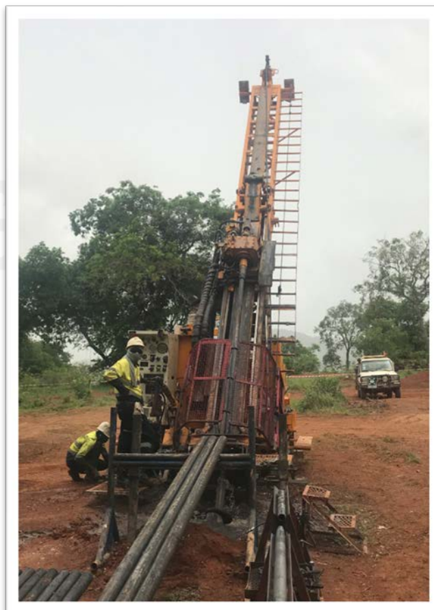
Figure 2: Diamond drilling underway at the Blaffo Gueto Prospect at Didievi in Côte d'Ivoire.
