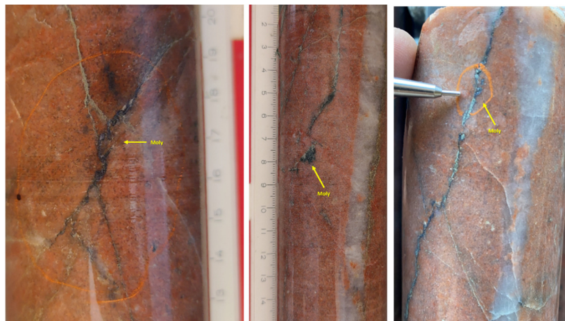
Figure 6: Molybdenite filling fractures.
