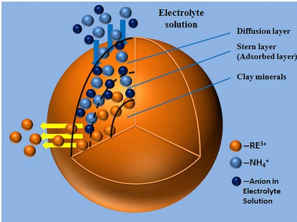
*Phase 1 met testwork demonstrated the initial basis with a simple salt desorption to exchange three NH<sub>4</sub><sup>+</sup> cations for one REE<sup>3+</sup> cation*
