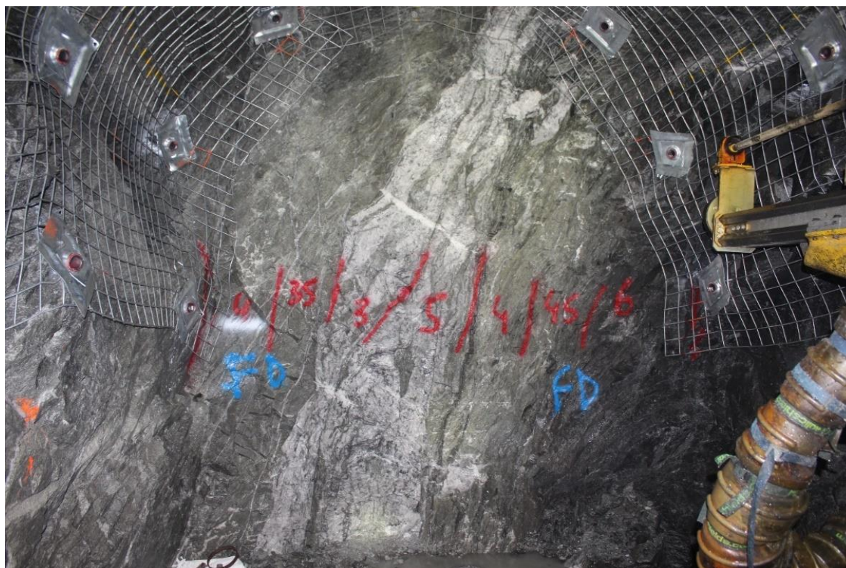
Figure 1: Easter Hollows development face, quartz vein lode grading 148 g/t with overall diluted face grading 48.6g/t
