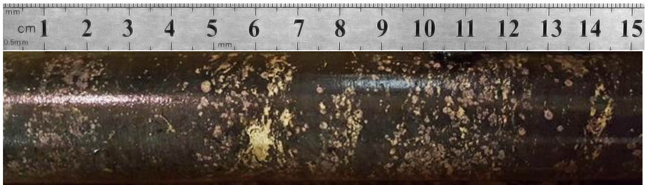
Figure 4: Photo of 36mm diameter Diamond Drill Core - Mineralisation style encountered in drill hole GRO20-02 at Green Mile. Biotite-Garnet-Amphibole alteration with 1-5% including visual chalcopyrite and minor pyrite, at 33.1m metres down.
