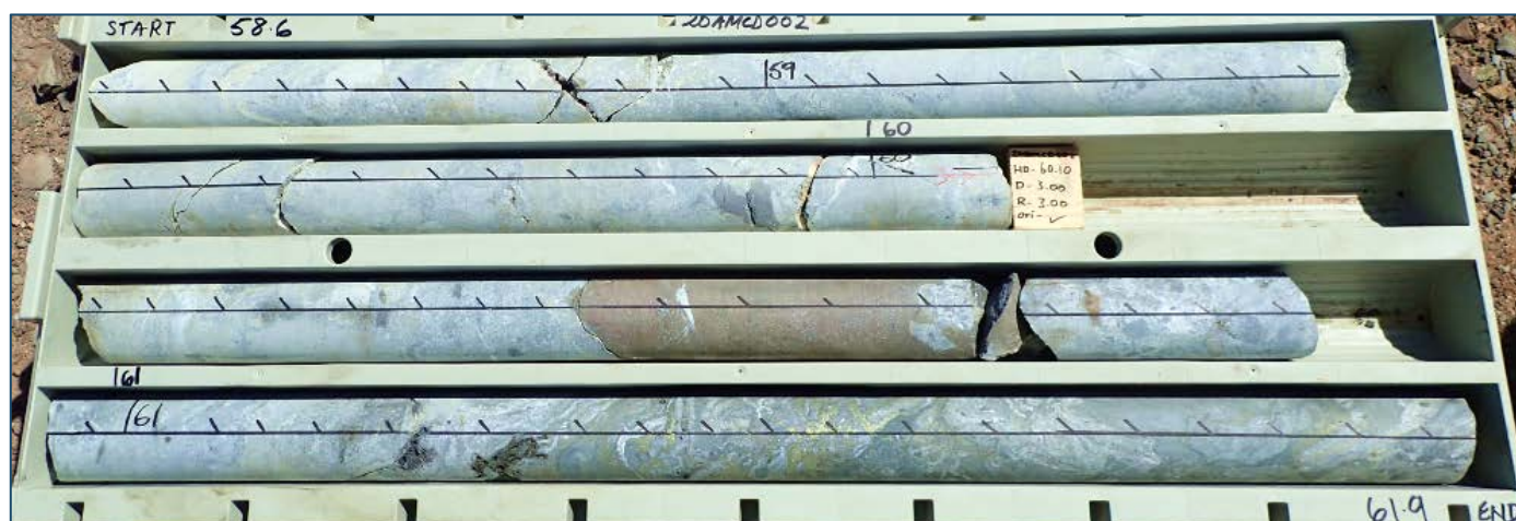
Figure 3: Massive sphalerite-galena mineralisation grading into a semi-massive to stringer zone within the upper chert horizon from 60.5m in diamond drill hole 20AMCD002.
