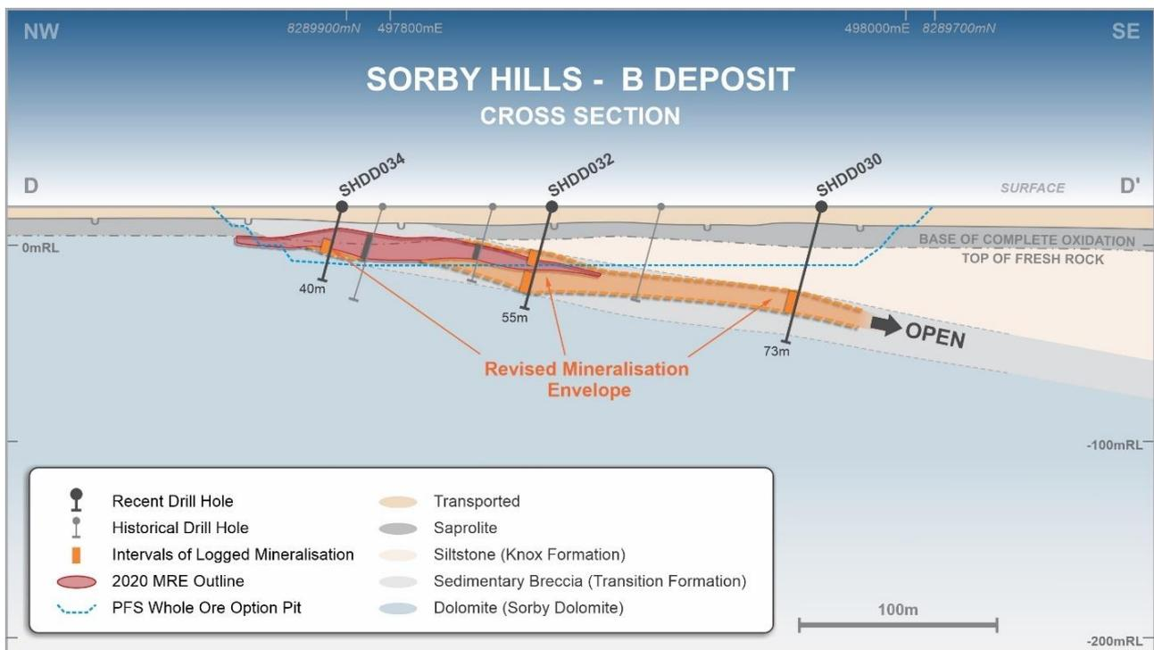
**Figure 5: Cross section through the B Deposit showing observed mineralisation in the newly completed drill holes SHDD030, SHDD032 and SHDD034 relative to the current Resource envelope and open pit design.**
