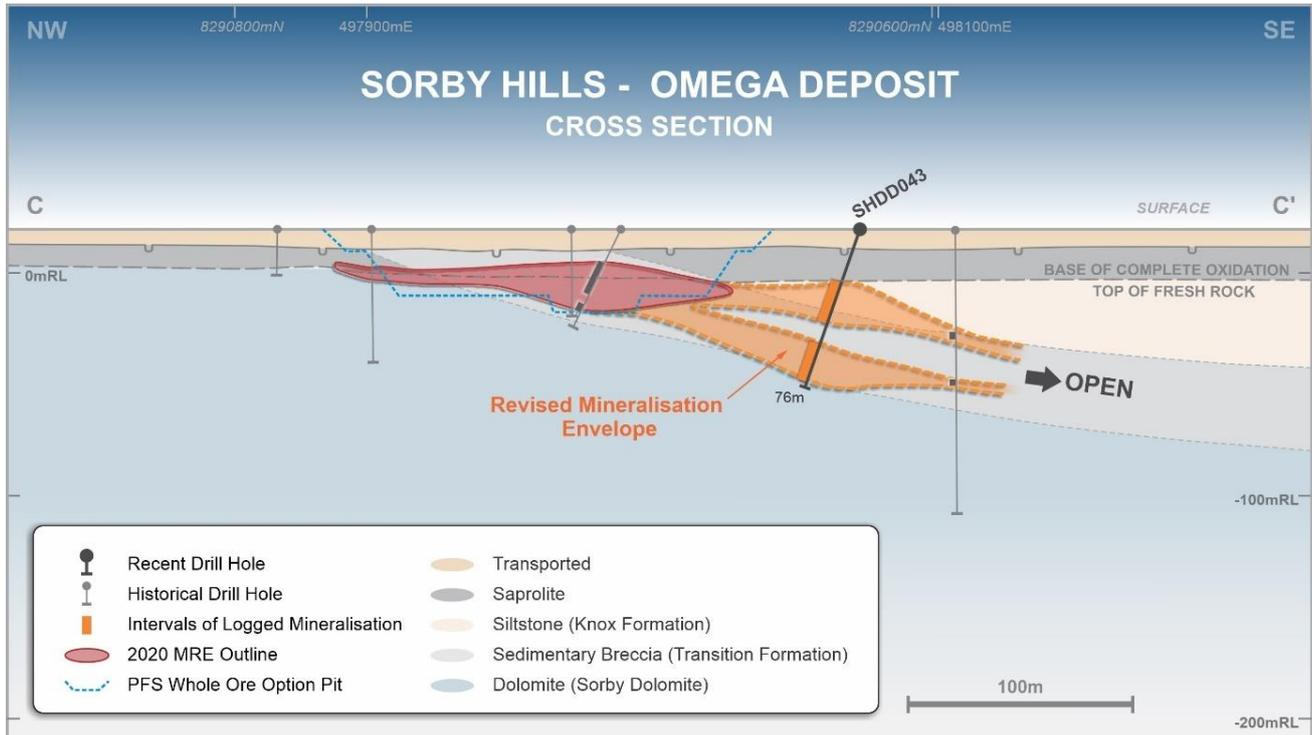
**Figure 3: Cross section [C-C'] through the southern portion of the Omega deposit showing observed mineralisation in the newly completed drill hole SHDD043 relative to the current Resource envelope and open pit design.**
