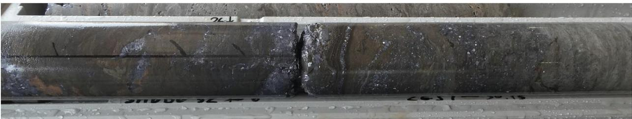
**Figure 6: Example of stratiform galena mineralisation intersected in SHDD032 at approximately 27m down hole depth.**
