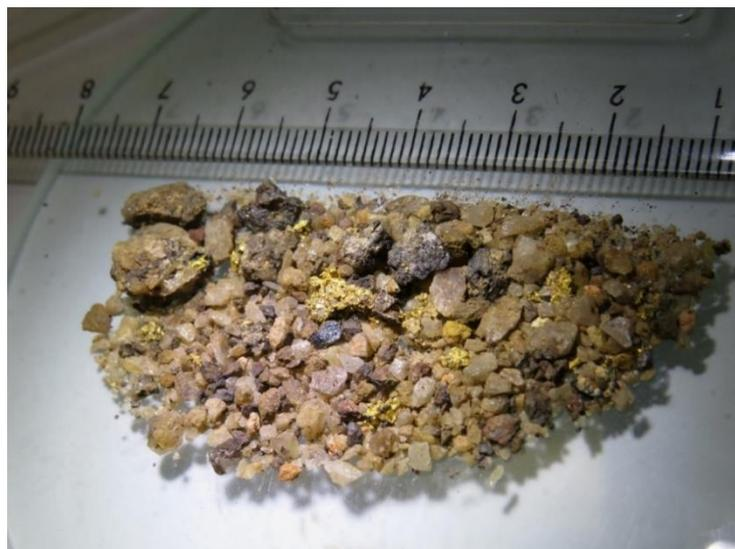
**Figure 3. Visible gold within ferruginised quartz breccia (drill chips; OGGRC266; 9-10m; original assay 830.4g/t Au with a repeat of 757.9g/t Au).**
