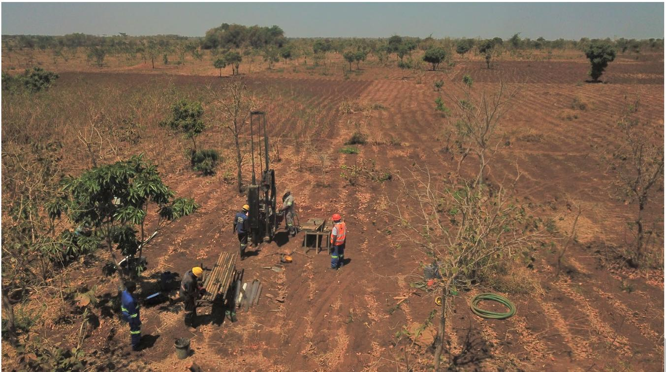
Figure 9: Drone photograph of the push-tube core rig in action at Kasiya.
