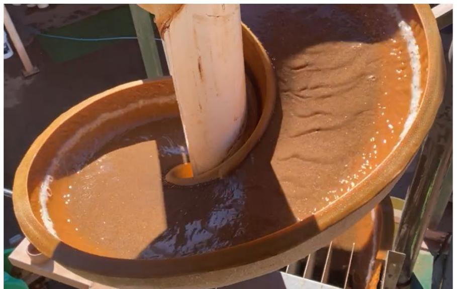
Figure 6 & 7. Left: Spiral processing of the sand fraction Right: Close-up of a working spiral processing the bulk-sample sand fraction from Kasiya
