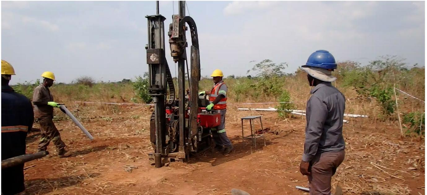
Figure 3. Push-tube core drilling at Kasiya.
