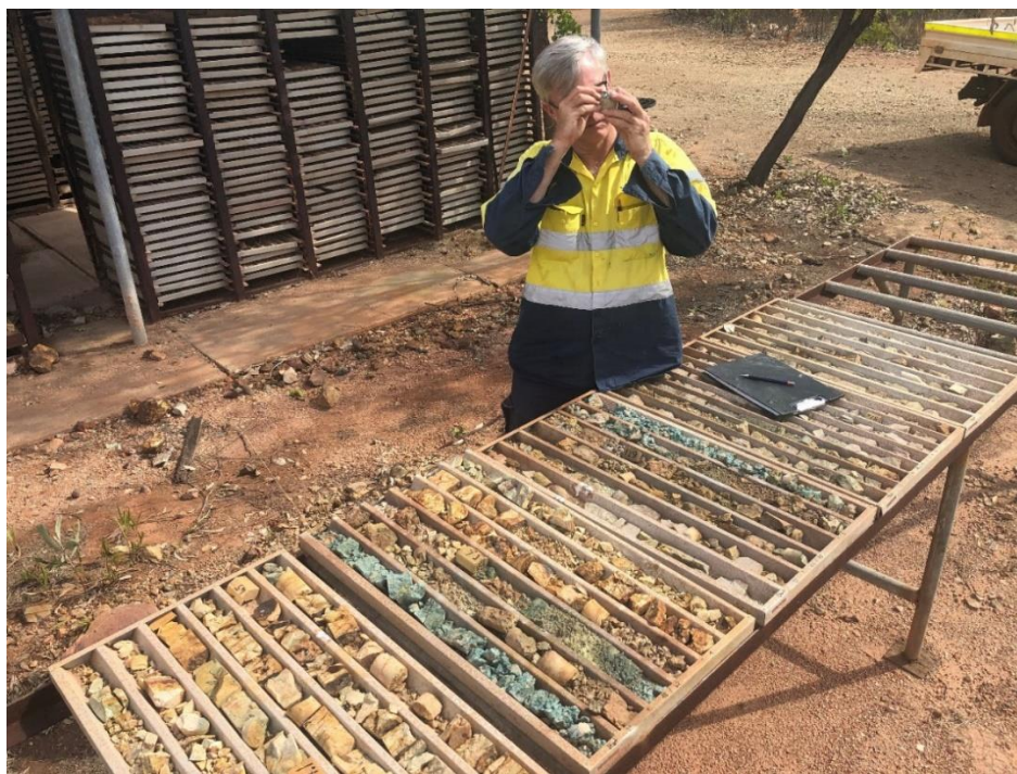
Figure 4. Drill core sampling at the Redbank Project at the onsite core shed
