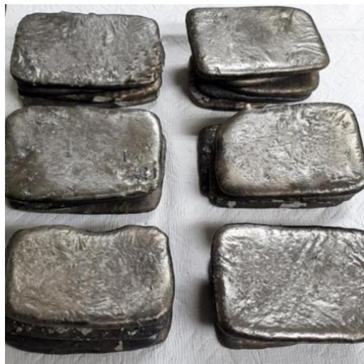
Figure 1: 200kg of FeNd metal alloy
