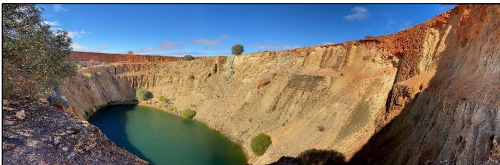
Figure 24 View of the southern wall of the Kohinoor pit clearly showing narrow BIF units
