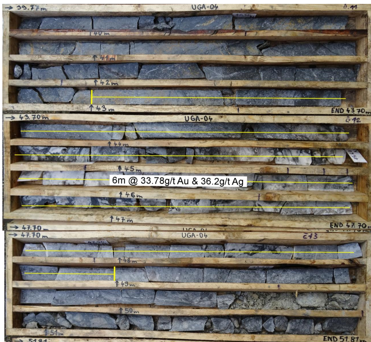
Figure 1: UGA-04 drill core; interval from 43m to 49m (down-hole) with assay grade 6m @ 33.78g/t Au and 36.2g/t Ag
