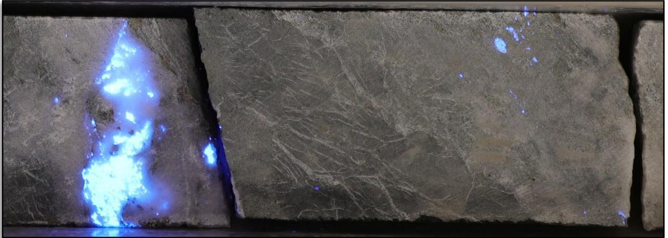
**Figure 5:** Mount Flora drill core under UV light showing scheelite (fluorescent blue colour) in silica-biotite altered basalt with quartz-carbonate-scheelite veining at 188.6m hole depth.
