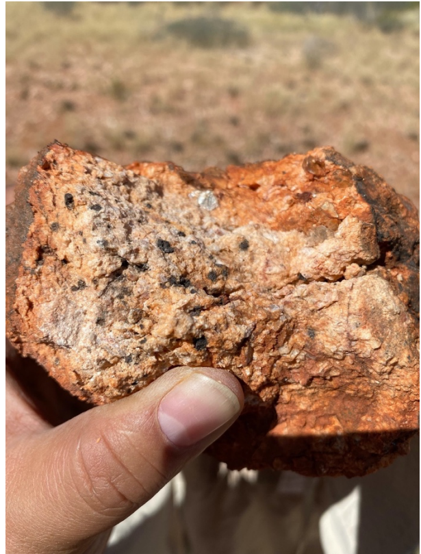
Figure 6: Tantalite identified in pegmatite rock chips.
