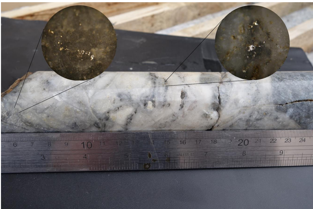
Figure 1: ~20cm wide zone containing multiple generations of drusy, fine grained, transparent to white to grey chalcedonic quartz-pyrite filled veins, some of which contain visible gold at 127.6-127.8m in UGA-30. Field of view of magnified images is ~4mm across (x40 magnification).
