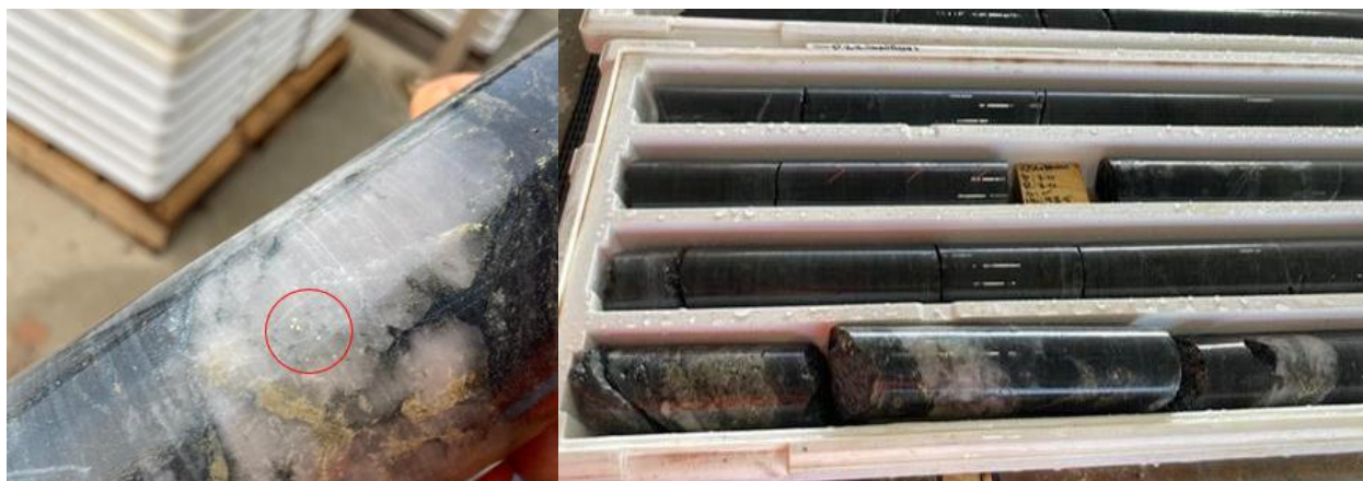
Figure 6: Deflector South West extensional drill core with quartz sulphide vein and visible gold
