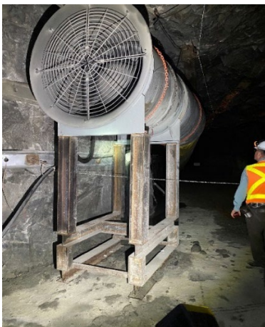
Photo 1 – Underground secondary fan
