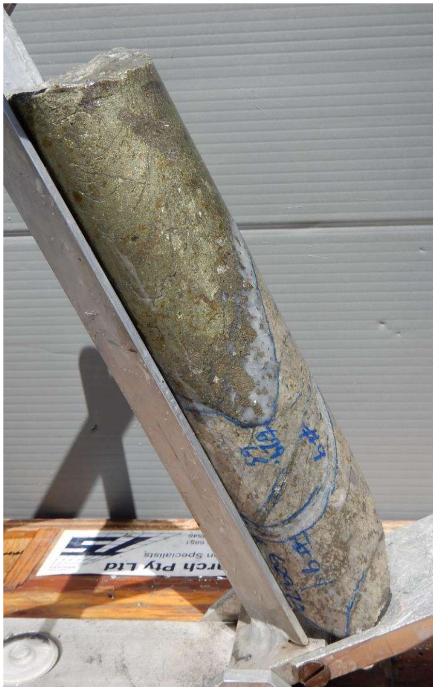
Fig 18 HQ Core photo hole 21CAEDD009, 629.65m HQ Core Photo in core frame oriented relative to actual drillhole surveyed position, CAE hole # 9, 629.6m ,view looking south, hole drilling 70 degrees to west. Large slug of chalcopryite and pyrite and quartz within intensely sericite altered and quartz pyrite veined , bleached diorite porphyry. 629m-630m assays 1m @ 1.60% Cu, 0.29 g/t Au, 23.1 g/t Ag, 7.97 % S
