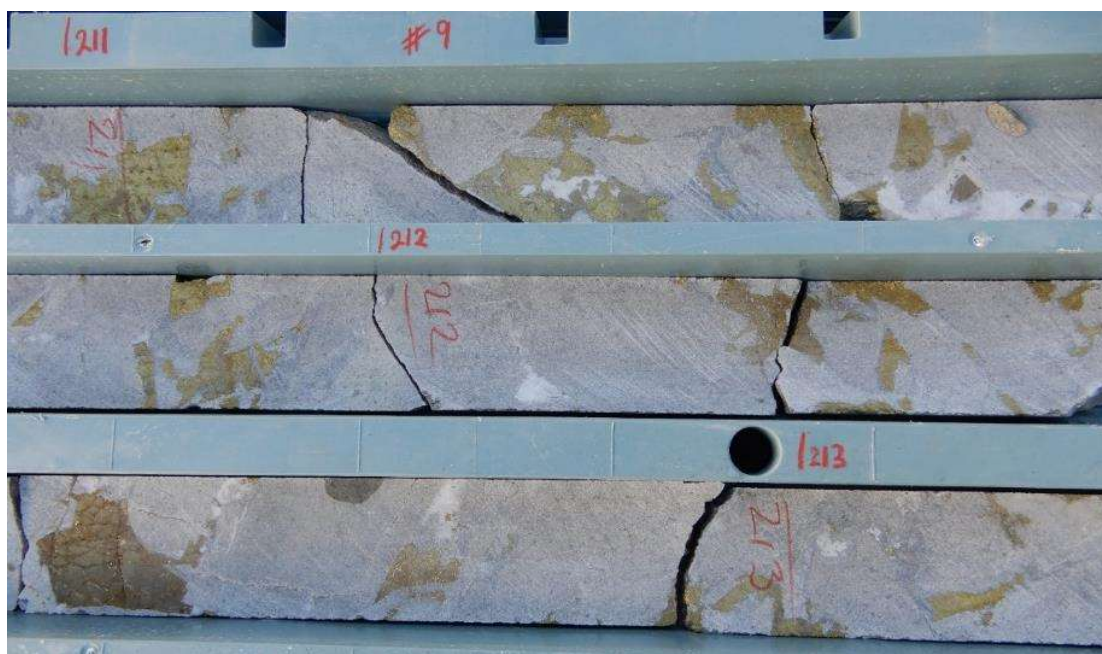
Fig 14 HQ Core photo hole 21CAEDD009, 211m-214m Chalcopyrite -pyrite infill in hydrothermal diorite dominated breccia. Primary zone 211m-214m assays 3m @ 2.78% Cu, 0.43 g/t Au, 41.8 g/t Ag, 6.24 % S
