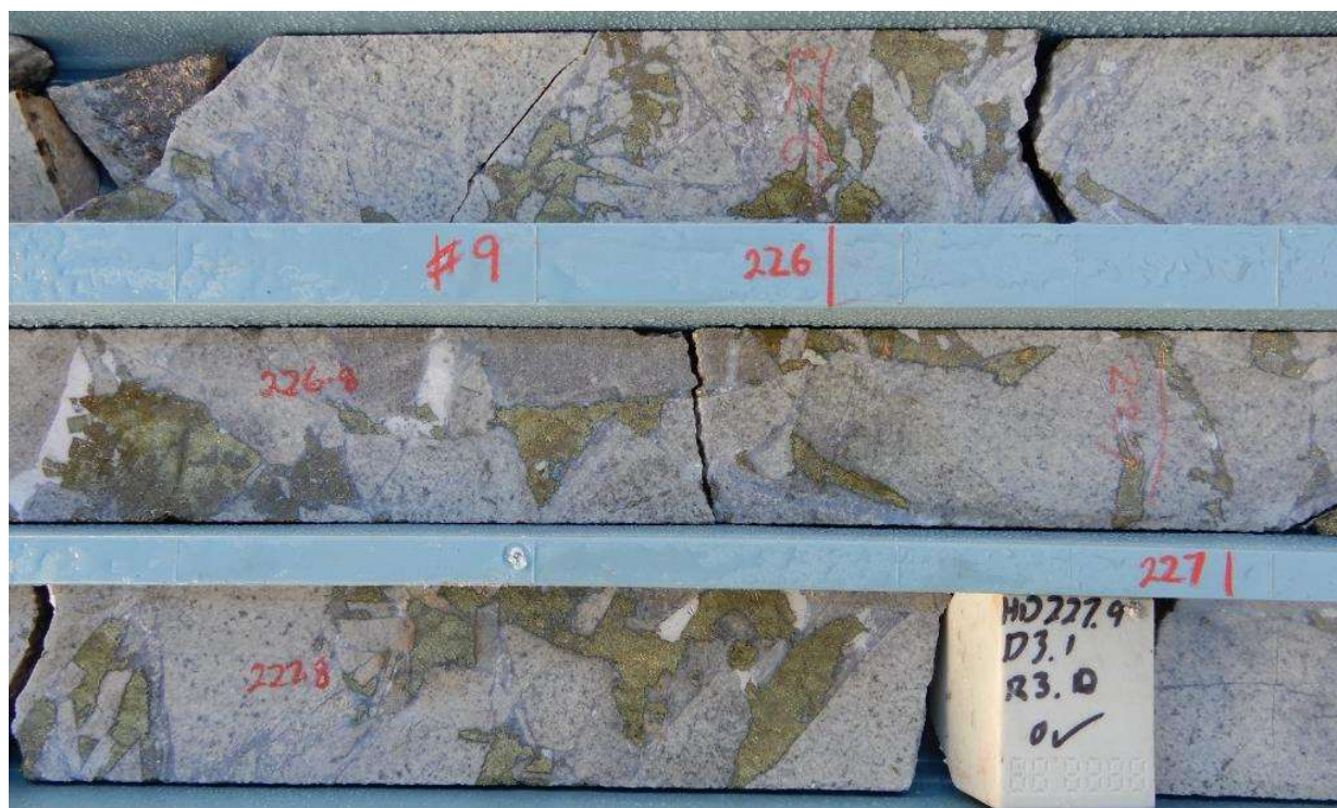
Fig 16 HQ Core photo hole 21CAEDD009, 225.7m-227.9m Chalcopyrite -pyrite calcite quartz infill in hydrothermal diorite dominated breccia. Primary zone 225m-228m assays 3m @ 3.84% Cu, 0.56 g/t Au, 43.5 g/t Ag, 6.46 % S
