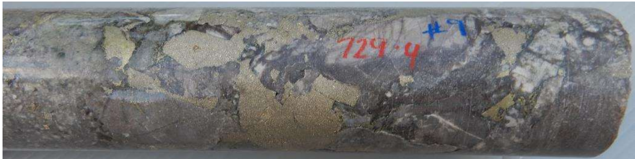
Fig 19 HQ Core photo hole 21CAEDD009, 729.4m Highly sulphidic clast supported breccia. Polymict clasts dominated by hornfels. Abundant pyrite, moderate chalcopryite infill. 729-730m assays 1m @ 0.27% Cu, 0.30 g/t Au, 8.4 g/t Ag, 8.5 % S.
