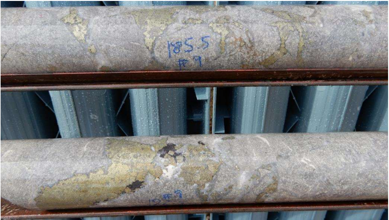
Fig 11 HQ Core photo hole 21CAEDD009, Two sections 182m (lower split), 185.5m (upper split), Chalcopyrite - pyrite sphalerite (black) infill in hydrothermal diorite dominated breccia. Primary zone 182m to 183m 1m @ 2.00% Cu, 2.04 g/t Au, 45.9 g/t Ag, 7.95 % S, 0.74% Zn . 185m to 186m 1m @ 1.32% Cu, 1.17 g/t Au, 32.8 g/t Ag, 5.49 % S .
