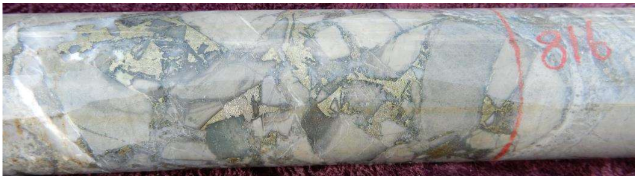
Fig 20 HQ Core photo hole 21CAEDD009, 816m Chalcopryite pyrite calcite quartz infill in hydrothermal sericite altered hornfels dominated breccia. Primary zone 815m-816m assays 1m @ 0.82% Cu, 0.19 g/t Au, 14 g/t Ag, 4.70 % S.
