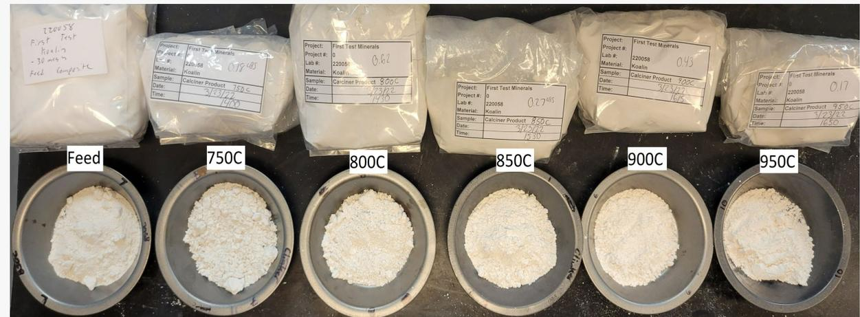
Flash calcined Gabbin hydroous kaolin tested by FLSmidth at various temperatures for suitability for Metakaolin
