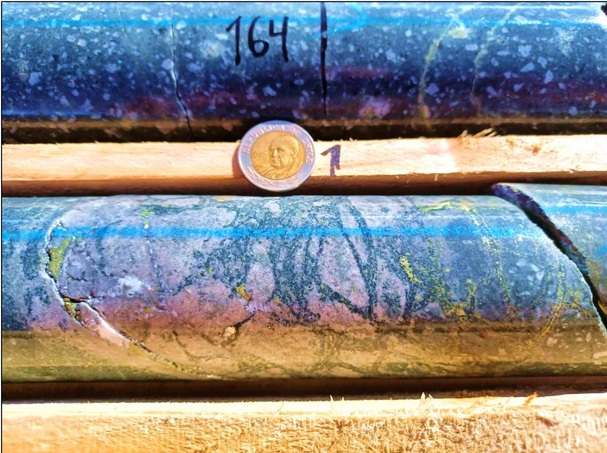
Figure 6: Crackle breccia hosted chalcopyrite mineralisation in drillhole CMLCD001, refer Appendix D (164 to 166m)<sup>1</sup>.
