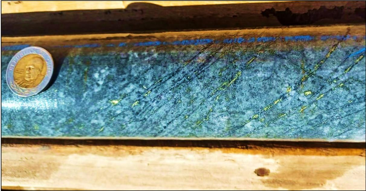
Figure 5: Sheeted vein hosted chalcopyrite mineralisation in drillhole CMLCD001, refer Appendix D (101 to 102m)<sup>1</sup>.
