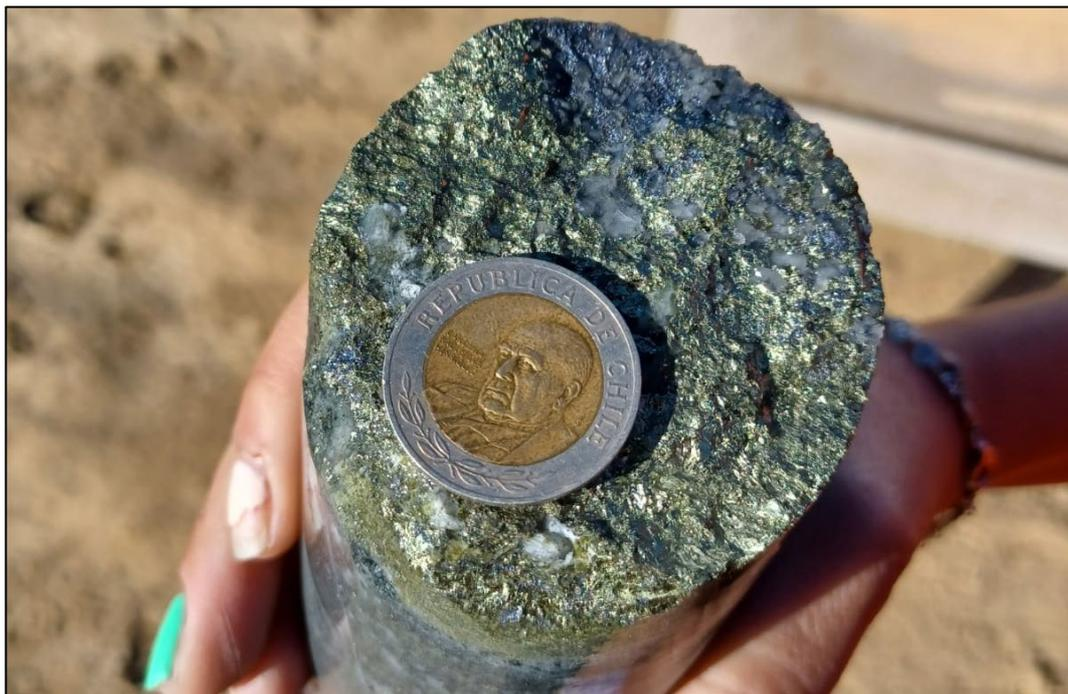
Figure 1: Core from CMLCD001 with Cu and Mo sulphides, refer Appendix D, (150-151m downhole)<sup>1</sup>.
