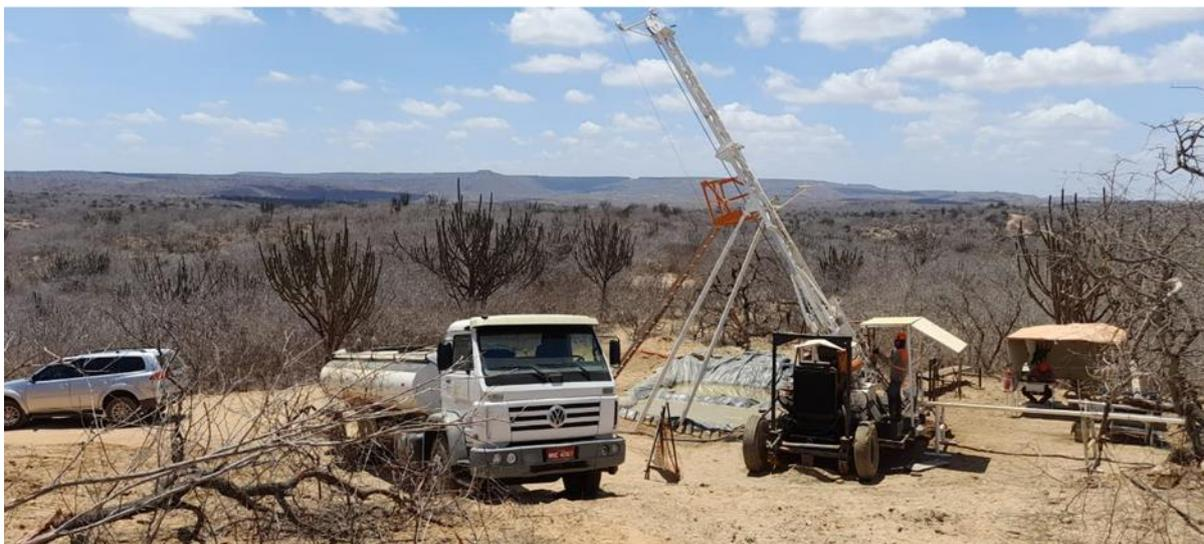
Figure 7 – Diamond drilling in progress at Borborema Gold Project
