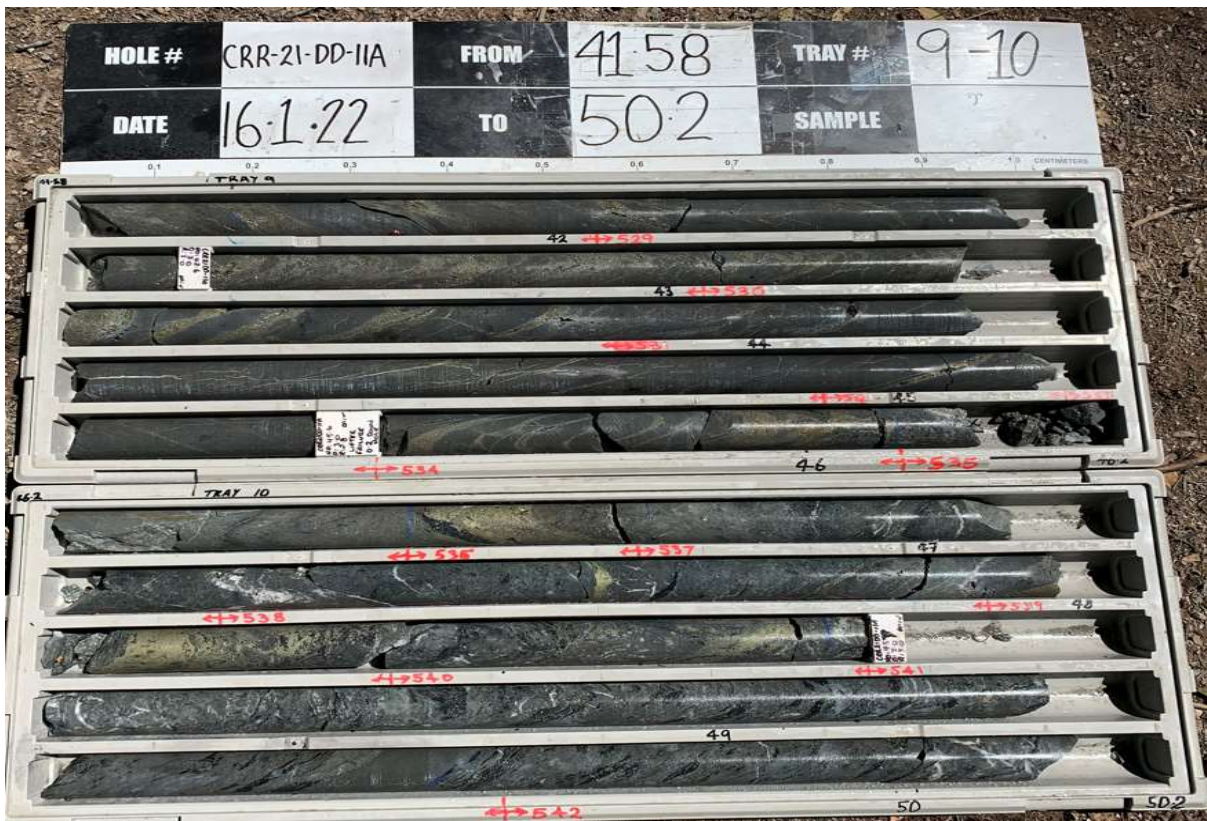
Figure 4: Detail of core with intervals of visible chalcopyrite and lesser pyrite, from first three rows of tray 10 in Figure 3 above that extend downhole from 46.2-48.7m. Top row RHS has portion of sample 536 (46.52-46.74m @ 3.30% Cu, 0.27% Zn, 0.019% Pb, 199.0g/t Ag, 0.02g/t Au;) and bottom row LHS has sample 539 (47.92-48.30m @ 6.89% Cu, 0.63% Zn, 0.01% Pb, 262g/t Ag, 0.02g/t Au), (Diamond drill hole CRR21DD_011A, Scale: NQ core 50mm diameter variety)
