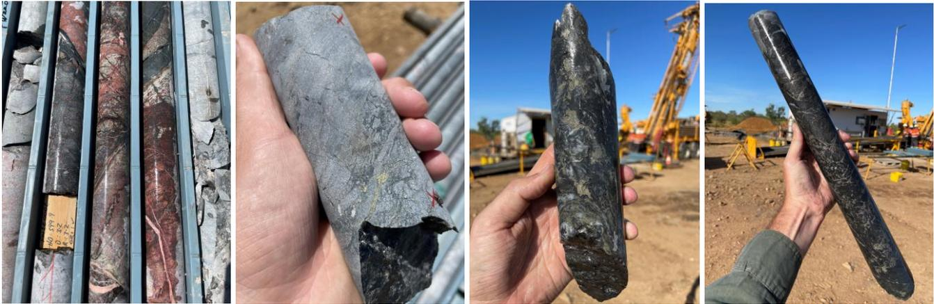
**Figure 1a:** Chlorite-haematite altered schist and haematite altered quartzite units with quartz veining (c. 400m depth); **1b** an irregular chalcocopyrite veinlet (c. 425m depth); **1c** quartz-pyrite veining in graphitic schist (c. 657m depth); **1d** pervasive pyrrhotite veining and laminations in graphitic schist (c. 660m depth).
