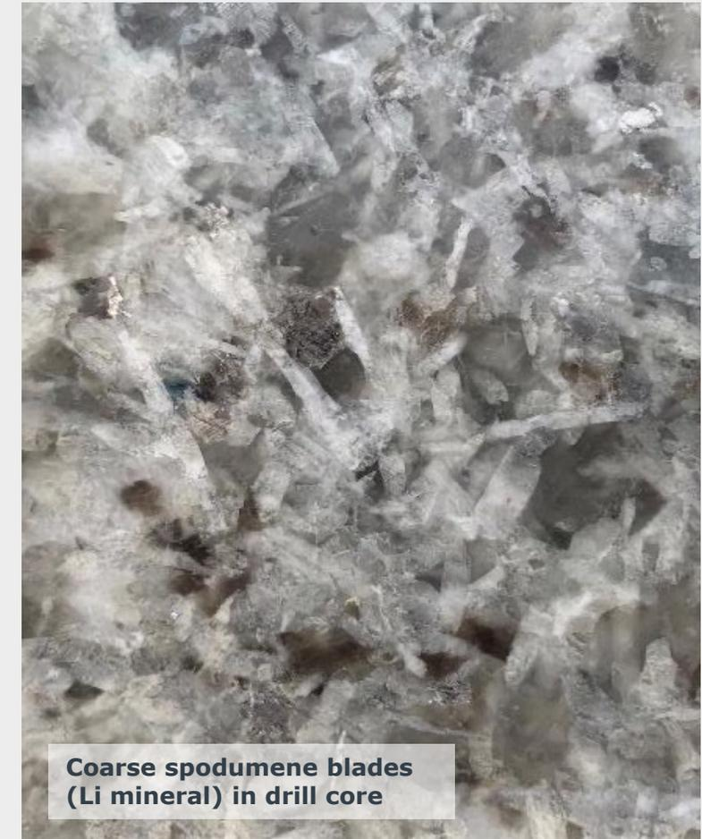
**Coarse spodumene blades (Li mineral) in drill core**
