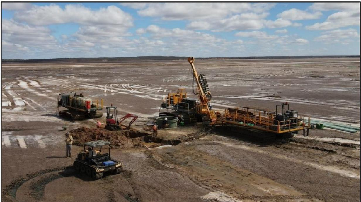
**Figure 1: Raglan Drilling’s lake rig sets up on first Sir Laurence diamond core hole**
