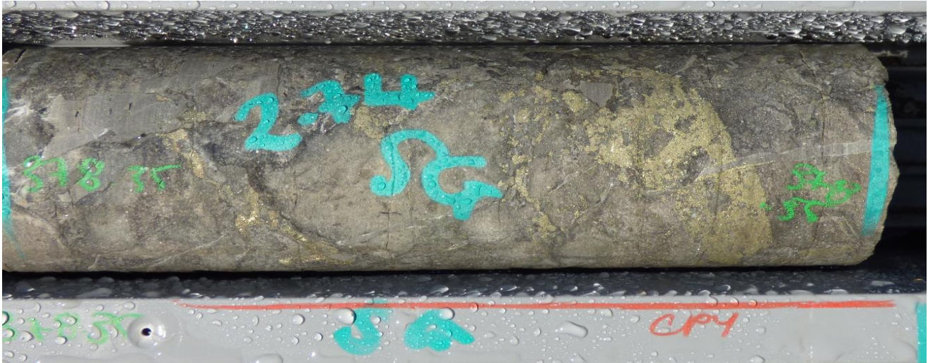
Figure 4: Drill core from WFDH375 378.7 metres showing chalcopyrite as matrix infill in the Walford Dolomite (sample is roughly 40m off the Fish River Fault)
