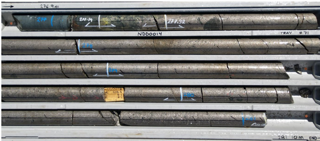
Figure 1. Massive sulphide intersected by NDD0014, which returned an average grade of 1.22% Ni.
