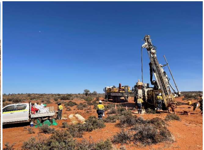
Figure 3: Aircore Samples (LHS) & Strike Aircore Rig in Operation (RHS)
