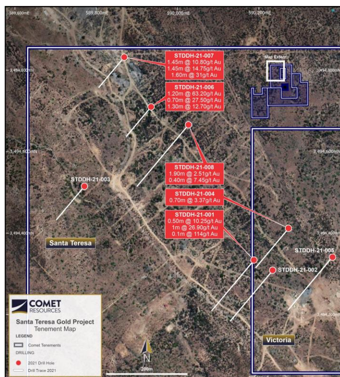
Figure 2: Plan view of drill collar locations and drill hole traces with key assay results indicated
