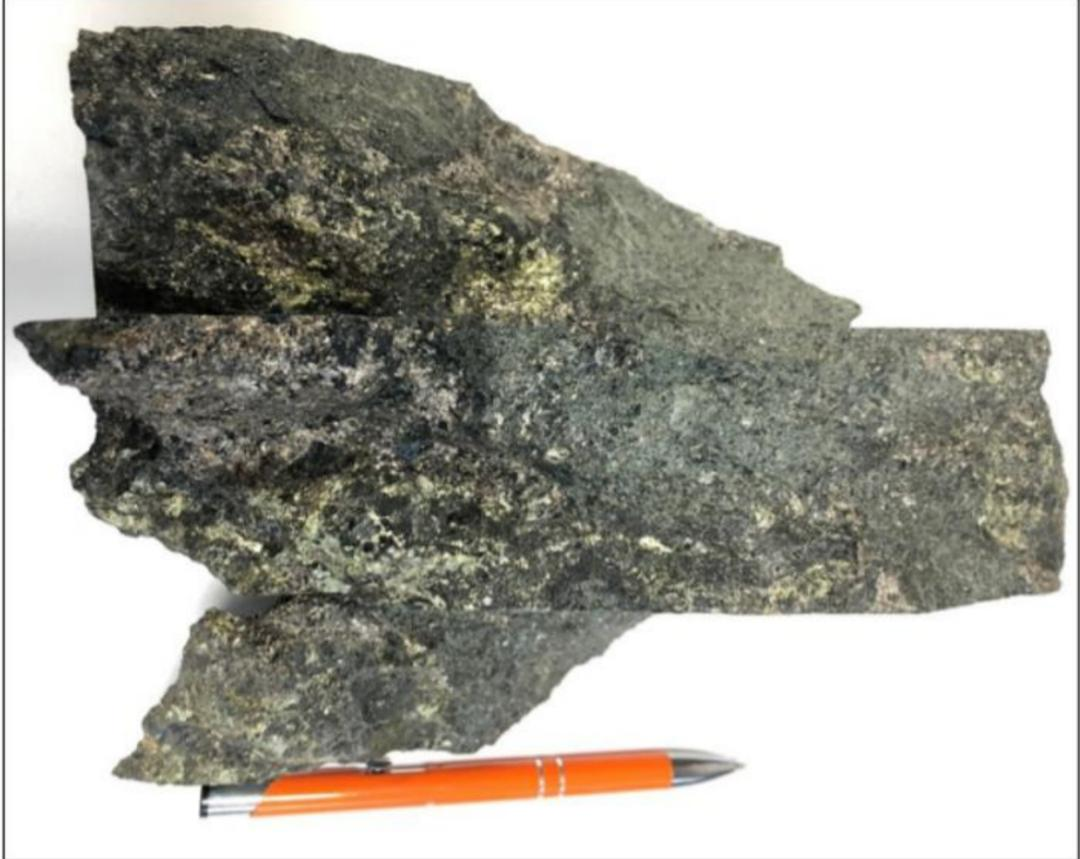
image:/photo: Mineralised pyroxenite with chalcopyrite, pyrrhotite and possibly pentlandite source: Azmiut Exploration
