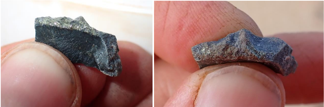
Figure 1: GRAC0042 at 79m. 2mm stringer of pyrrhotite (dark brown) with minor chalcopyrite (bright yellow).
