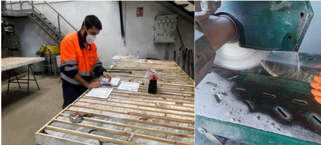
Figure 2. Drill core logging and drill core cutting for the sampling process at Finx Sn-W mine.
