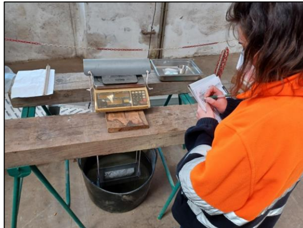
Figure 4. Rock density measurements from drill core is carried out systematically at San Finx.
