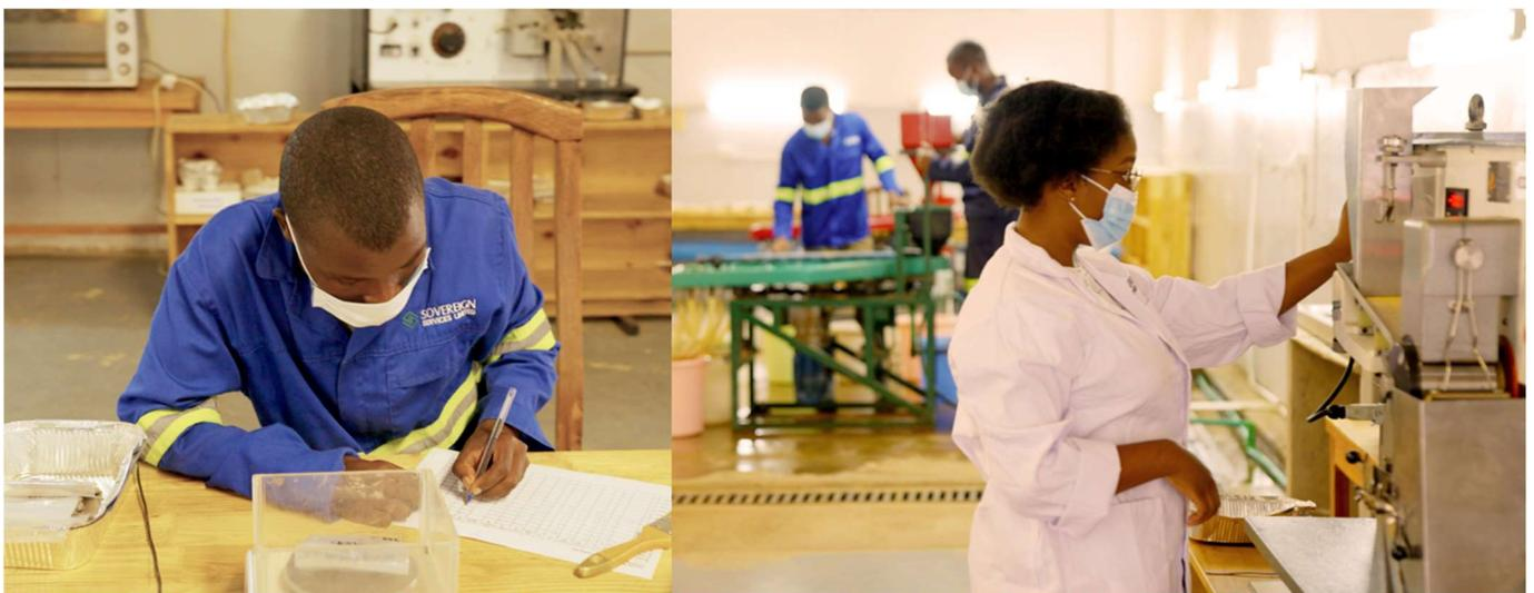
Figures 3 & 4: Recording sample weights (L) and conducting magnetic separation (R) at the Company's laboratory in Lilongwe
