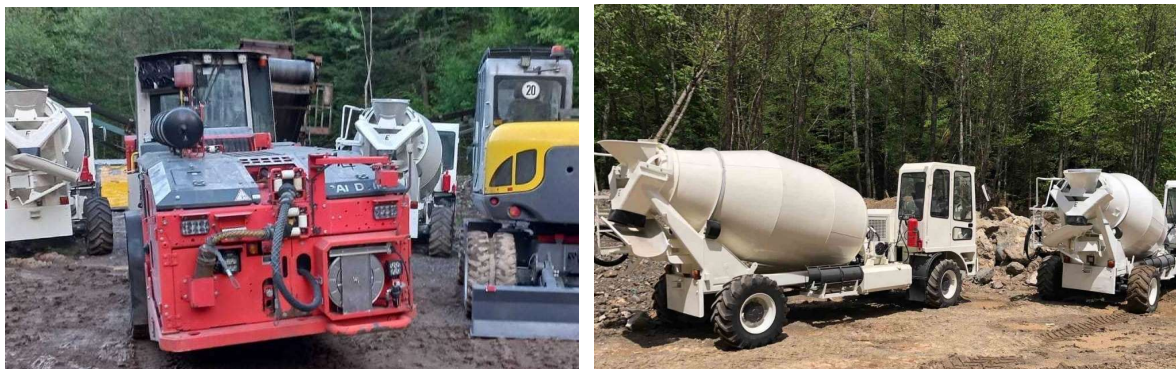
Underground concrete mixer trucks, jumbo & excavator will be used during the first phase of mining for decline construction
