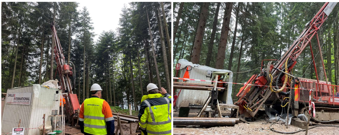
Drillex International diamond core drilling rigs operating near Rupice
