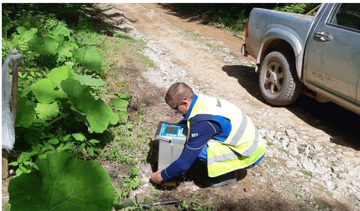
Enerson Engineering performing the ground gravity survey near the SP1 target
