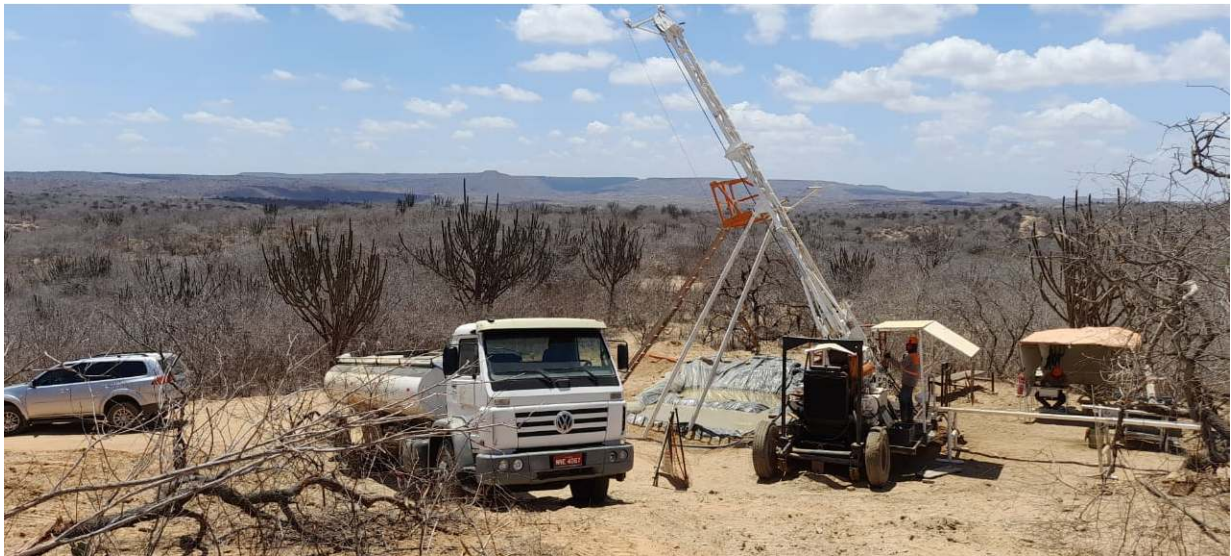
Figure 1 – Diamond Drilling at Borborema Gold Project
