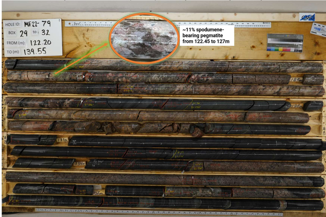
Figure 7: White pegmatite hosts approximately 10% of fine to medium, white-grey, spodumene crystals intersected from 122.45 to 127 metres depth in Hole MF22-79 (Hole 20). Close-ups illustrate significant spodumene mineralisation.
