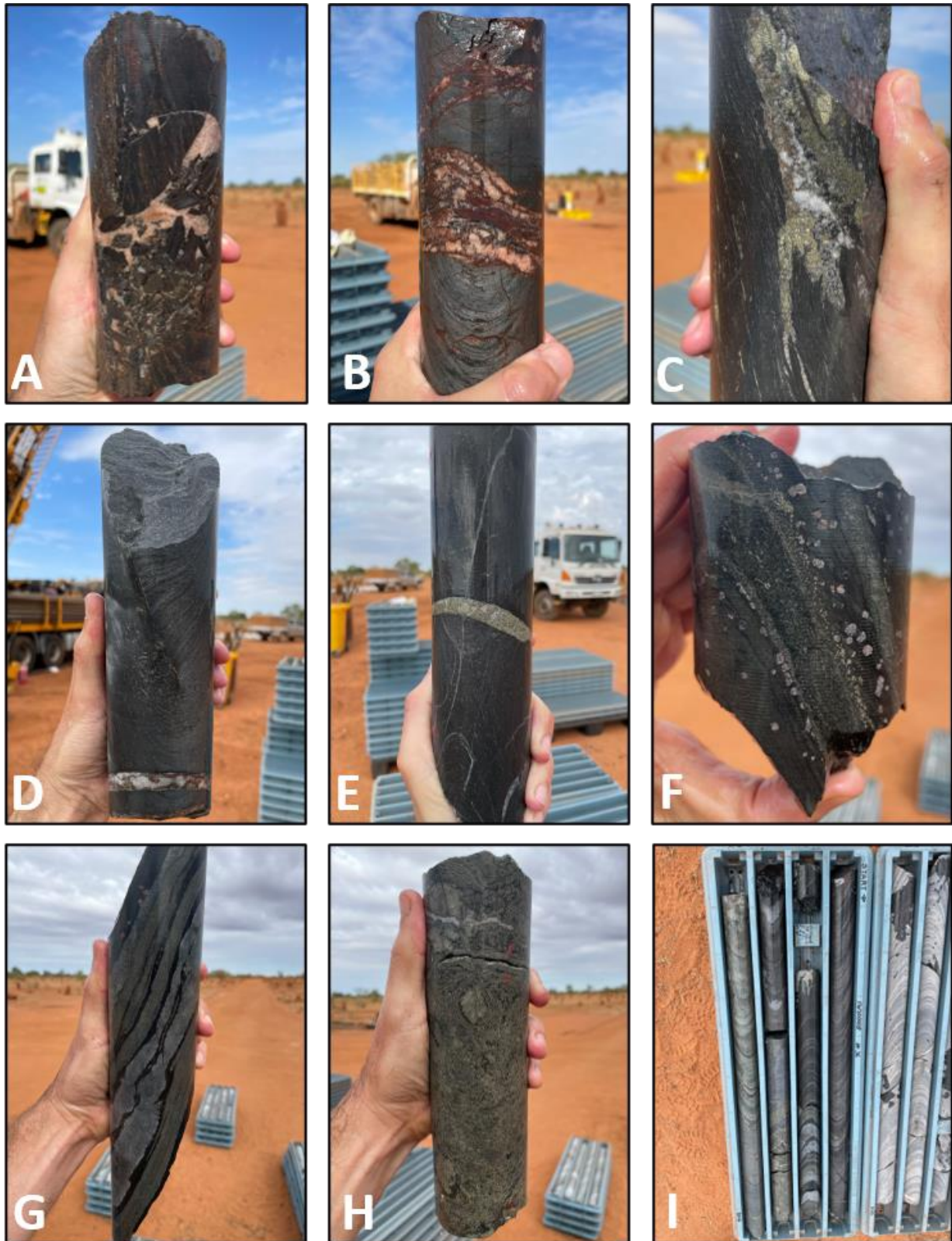
Figure Ap2(A): Core photo collage showing the progression of geology, alteration and veins down FW220008, including: A) quartz-(haematite) matrix in breccia zone within mica schist at 221m, B) quartz-haematite and quartz veinlets cutting mica schist at 234m, C) pyrite occurring as laminations parallel to foliation in mica schist and pyrite-quartz-haematite-(chalcopyrite) veins at 240m, D) abundant pyrite in mica schist foliations cut by 1cm wide quartz-haematite-pyrite-(chalcopyrite) vein at 251m, E) quartz-pyrite vein cutting pyritic shale-schist at 253m, F) laminated and pyritic shale with very fine grained to coarse grained garnets that show variable overprinting by quartz-(pyrite) at 286m, G) laminated and pyritic shale-siltstone with very fine grained to coarse grained garnets that show variable overprinting by quartz-(pyrite) at 286.5m, H) 50cm-wide massive pyrite zone at 287m within strong silicification, and I) core tray image including Photo H of massive pyrite within strong silicification at c. 287m.
