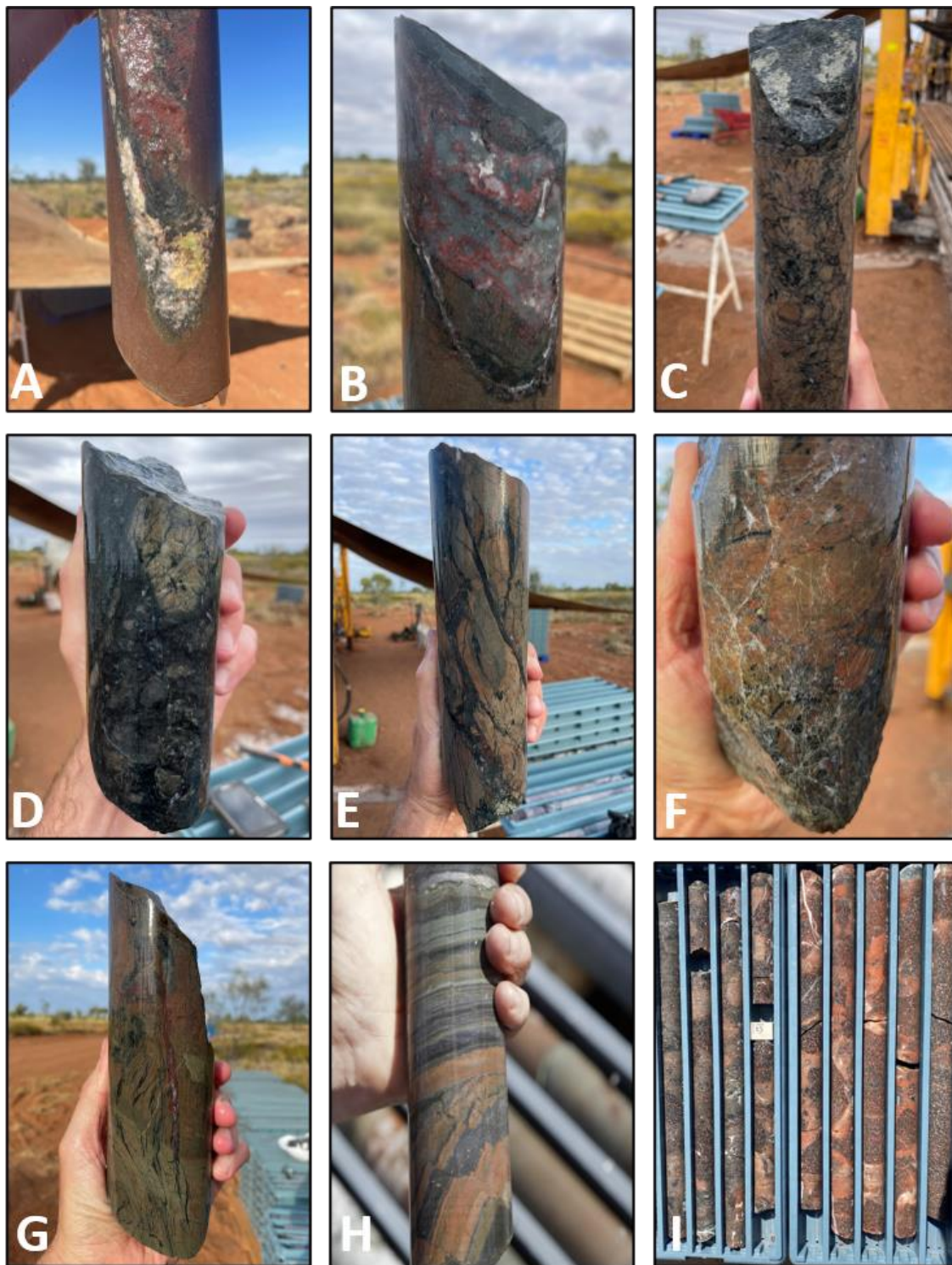
Figure Ap1(A): Core photo collage showing the progression of geology, alteration and veins down FW220004, including: A) quartz-calcite-epidote-chlorite-(haematite) veining in fine-grained sandstone at 216m, B) quartz-haematite-chlorite veining in sandstone at 565m, C) brecciated and altered siltstone with abundant pyrite and trace chalcopyrite on fracture surfaces at 595m, D) 30cm wide breccia zone with haematite-quartz-chlorite-epidote and trace fluorite with disseminated rare-trace pyrite-chalcopyrite at 599m; breccia clasts are fractured suggesting multiphase fluid flow, E) veined and brecciated siltstone at 602.5m with chlorite-quartz-haematite-fluorite-pyrite, F) veined and brecciated siltstone with chlorite-quartz-haematite-fluorite-pyrite-chalcopyrite at 604m, G) haematite-quartz-chlorite-pyrite veined siltstone at 618m, H) faulted siltstone at 670m, and I) brecciated and veined volcanics with haematite alteration of feldspar and quartz hosting minor pyrite at 713m.
