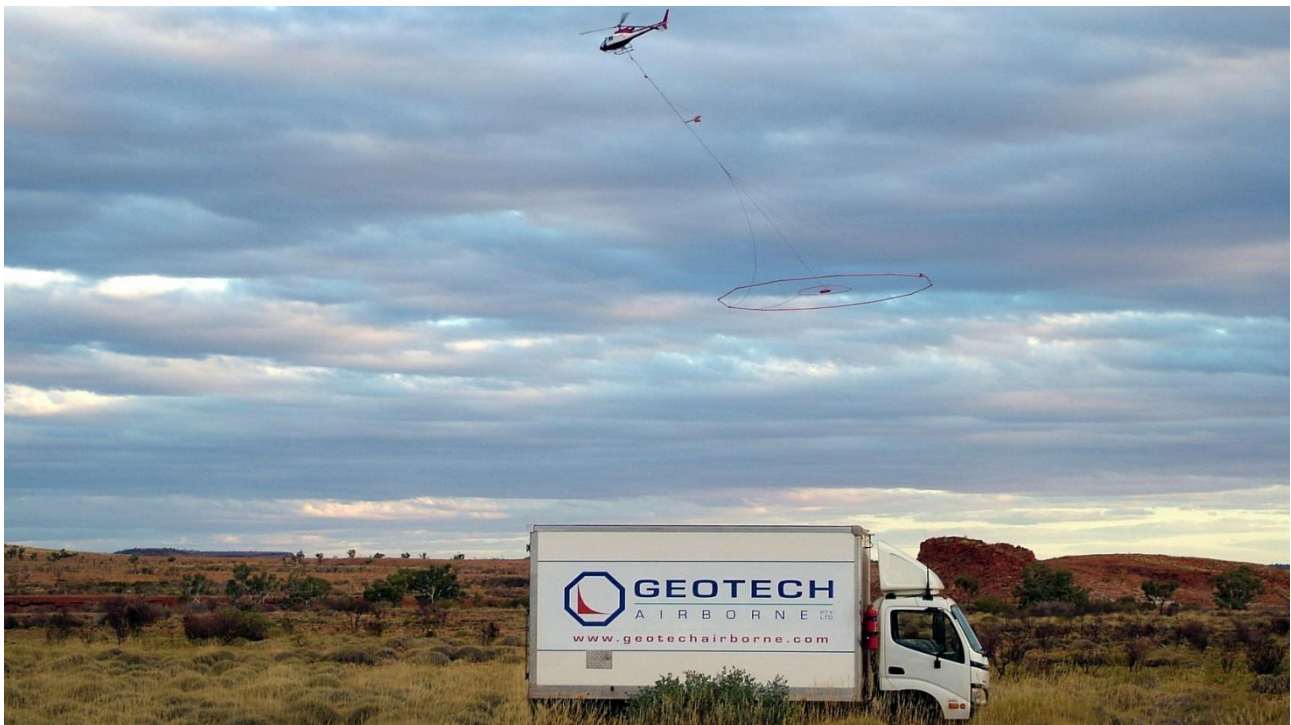
Figure 1 – Image courtesy of UTS (Geotech) of the VTEM MAX system in operation
