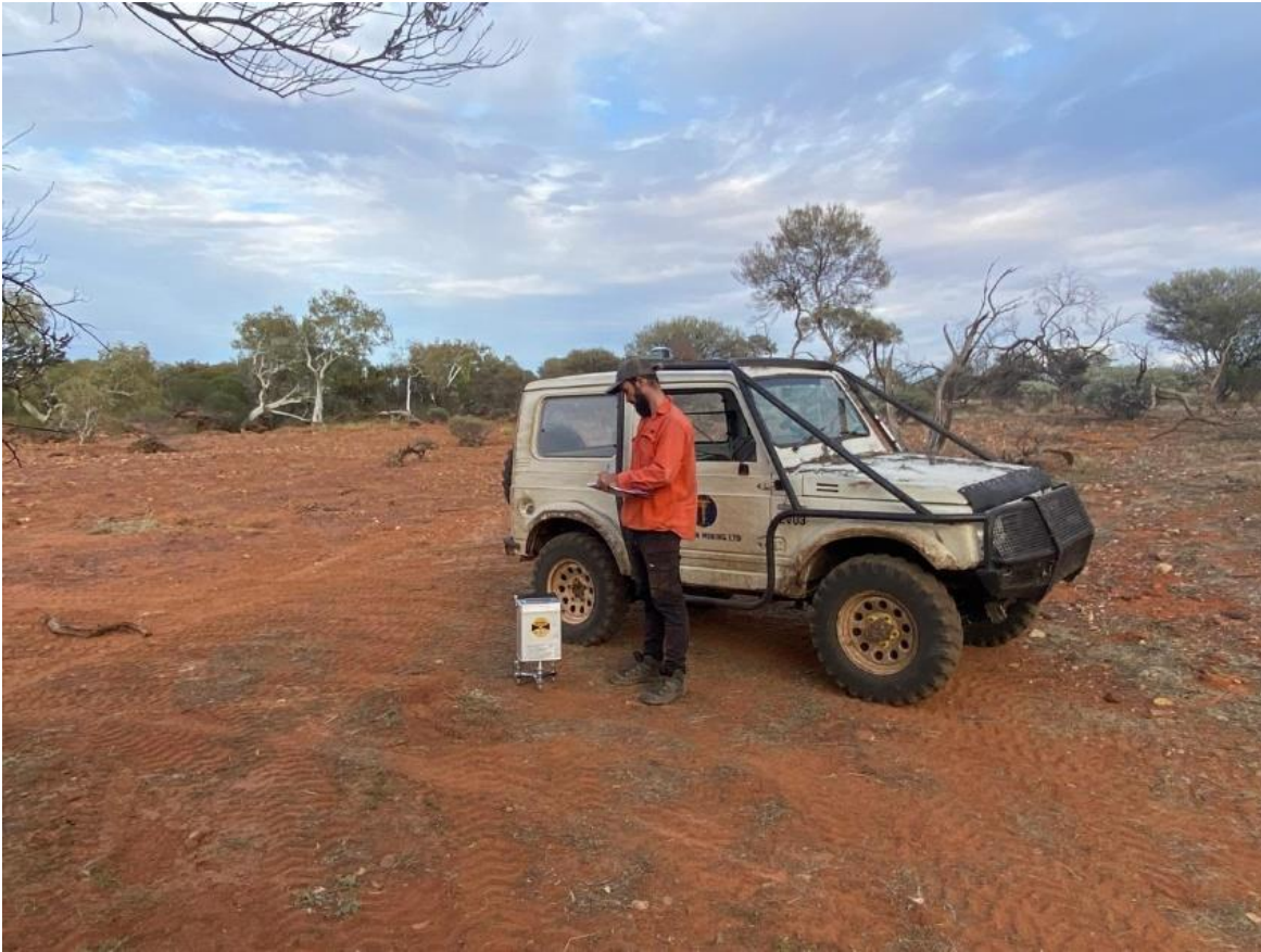
Figure 4 – Atlas Geophysics, May 2022 Ground gravity survey (1km x 1km station spacing)
